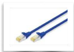
DK-1644-A-100/B CAT 6A S-FTP patch cord, Cu, LSZH AWG 26/7, length 10 m, color blue
