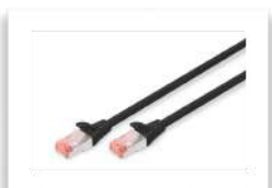
DK-1644-050/BL CAT 6 S-FTP patch cord, Cu, LSZH AWG 27/7, length 5 m, color black
