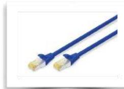
DK-1644-A-005/B CAT 6A S-FTP patch cord, Cu, LSZH AWG 26/7, length 0.5 m, color blue
