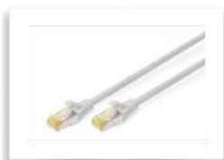
DK-1644-A-070 CAT 6A S-FTP patch cord, Cu, LSZH AWG 26/7, length 7 m, color grey
