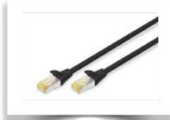
DK-1644-A-020/BL CAT 6A S-FTP patch cord, Cu, LSZH AWG 26/7, length 2 m, color black
