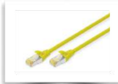
DK-1644-A-005/Y CAT 6A S-FTP patch cord, Cu, LSZH AWG 26/7, length 0.5 m, color yellow
