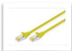
DK-1644-A-050/Y CAT 6A S-FTP patch cord, Cu, LSZH AWG 26/7, length 5 m, color yellow
