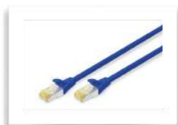
DK-1644-A-070/B CAT 6A S-FTP patch cord, Cu, LSZH AWG 26/7, length 7 m, color blue
