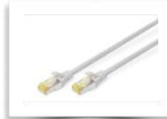
DK-1644-A-010 CAT 6A S-FTP patch cord, Cu, LSZH AWG 26/7, length 1 m, color grey
