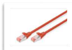
DK-1644-050/R CAT 6 S-FTP patch cord, Cu, LSZH AWG 27/7, length 5 m, color red
