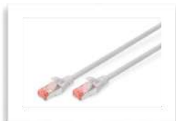
DK-1644-150 CAT 6 S-FTP patch cord, Cu, LSZH AWG 27/7, length 15 m, color grey
