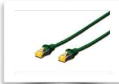
DK-1644-A-010/G CAT 6A S-FTP patch cord, Cu, LSZH AWG 26/7, length 1 m, color green
