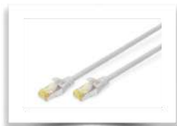
DK-1644-A-150 CAT 6A S-FTP patch cord, Cu, LSZH AWG 26/7, length 15 m, color grey
