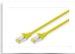
DK-1644-A-030/Y CAT 6A S-FTP patch cord, Cu, LSZH AWG 26/7, length 3 m, color yellow
