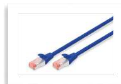
DK-1644-030/B CAT 6 S-FTP patch cord, Cu, LSZH AWG 27/7, length 3 m, color blue
